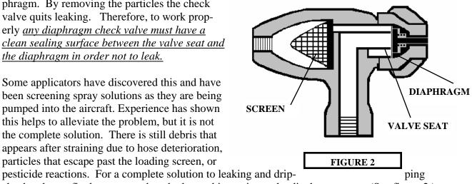
check valves a final screen needs to be located just prior to the diaphragm area. (See figure 2.)
