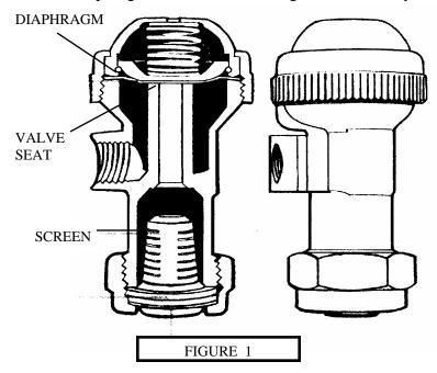
uses. The parts of a check valve the operator needs to be familiar with are the valve seat, the diaphragm, and the cap (Please refer to figure. 1). As the spray valve is opened the pesticide solution pressurizes the outer ring causing the spring in the cap to compress; usually occurring at 15 psi., allowing the pesticide solution to flow through the valve seat and out the spray tip.
